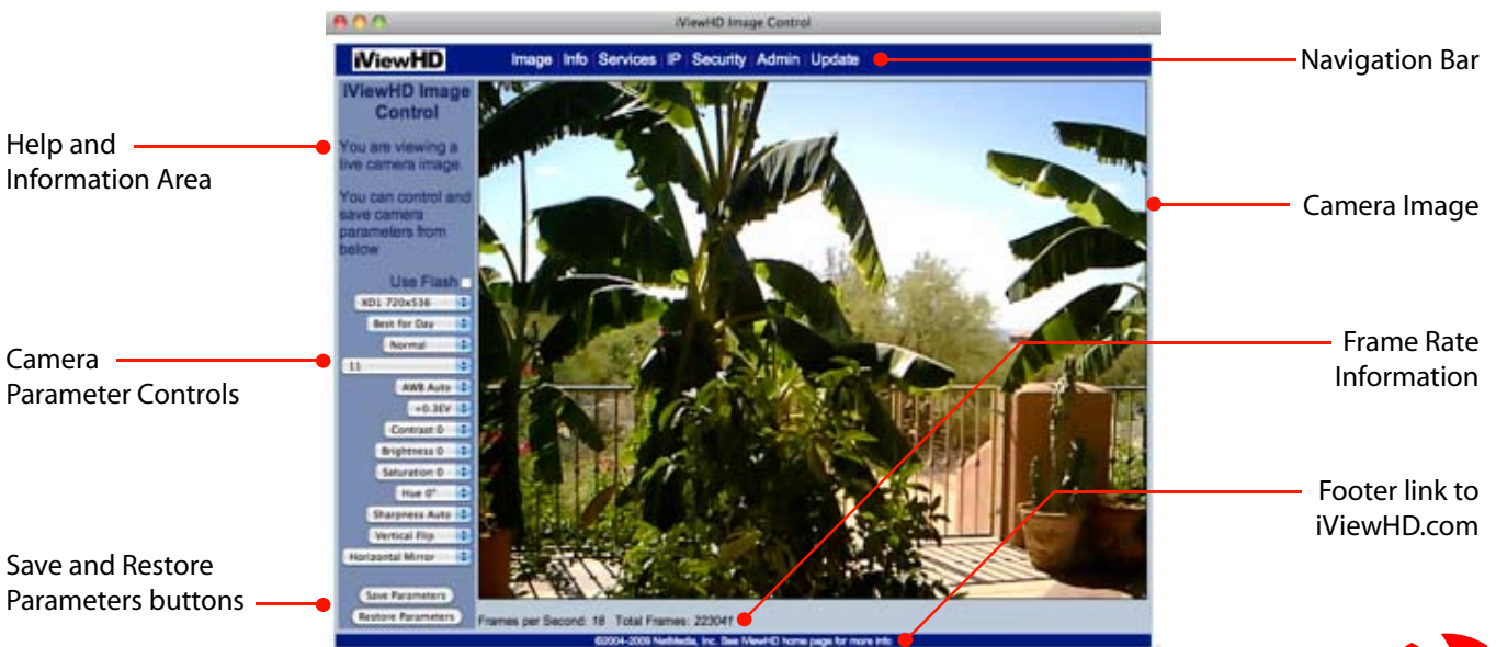
Figure 3 - iViewHD Image page for viewing camera output and adjusting, saving, and restoring camera settings.
