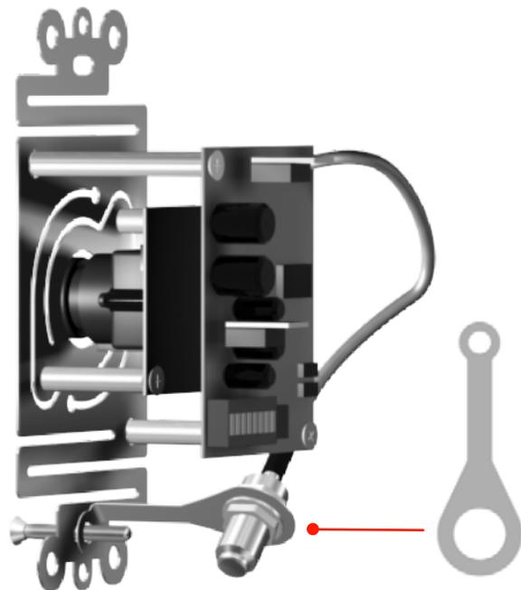
Figure 4 - Grounding the camera through the bracket with a grounded coax
