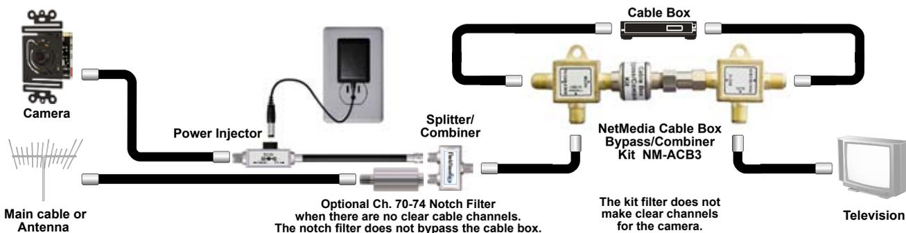
Figure 5 - Bypassing a digital or analog cable box and recombining to a single coax input on the TV. The kit's filter removes any conflict on channel 3 or 4. Switch TV from the cable box to the camera channel.
