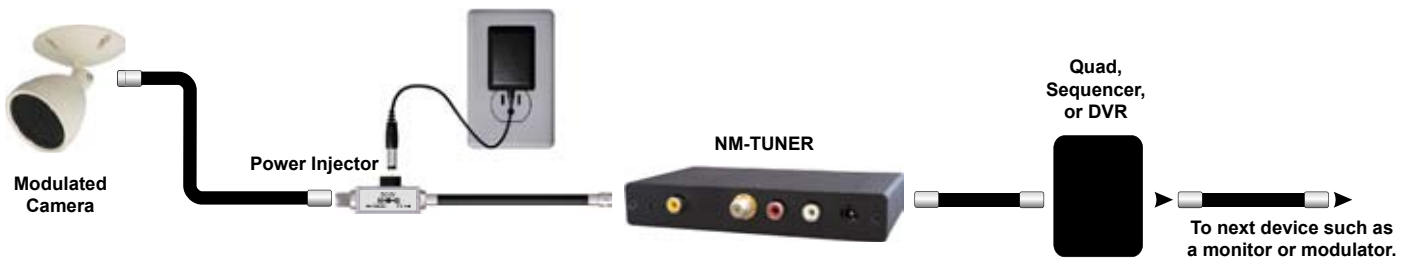
Figure 2 - Connecting the tuner to a modulated camera and video device such as a Quad, Sequencer, or DVR.
