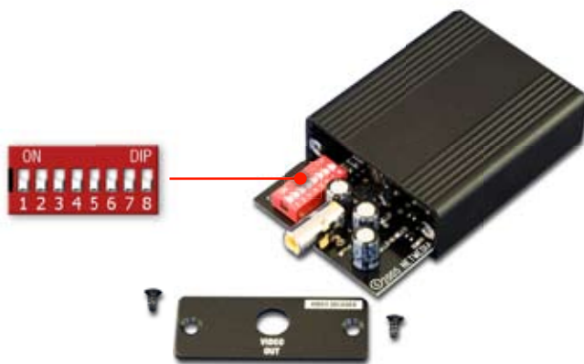
Figure 5 - UTP Decoder DIP Switches. Default of all OFF works for most installations. If necessary, start with #1 and turn more ON as the cable length increases; turn them all ON for the longest distance, 1000 feet.
