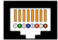
Figure 4 - T-568A standard straight-through wiring diagram. Connect pin 1 of each plug together with the same wire. Repeat for all the corresponding pins.
