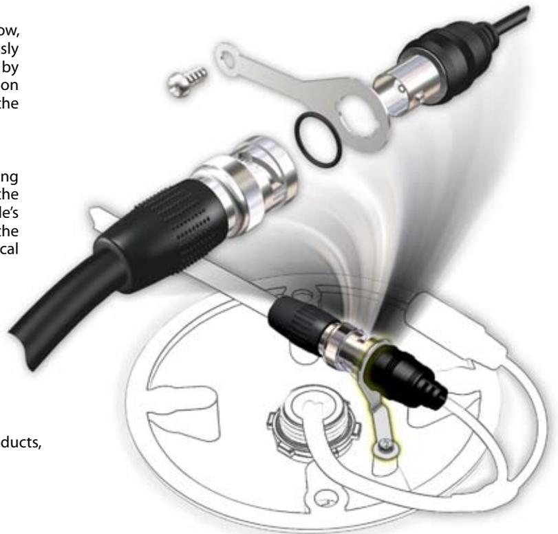
Figure 4 - Grounding the camera through the base with a grounded coax (base may vary according to model).
