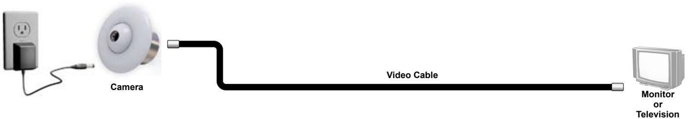
Figure 1 - Connecting the camera to a security monitor or standard television. Use the TV's composite RCA Video In jack and view through its video or line input. The picture will not be available on a channel.
