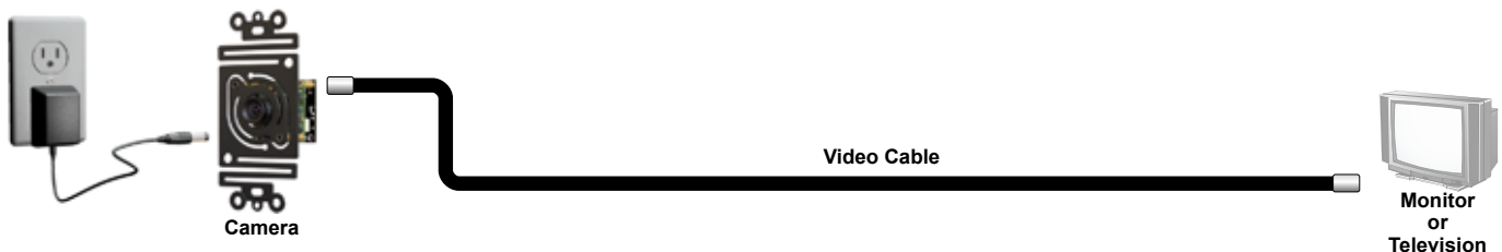
Figure 1 - Connecting the camera to a security monitor or standard television. Use the TV's composite RCA Video In jack and view through its video or line input. The picture will not be available on a channel.
