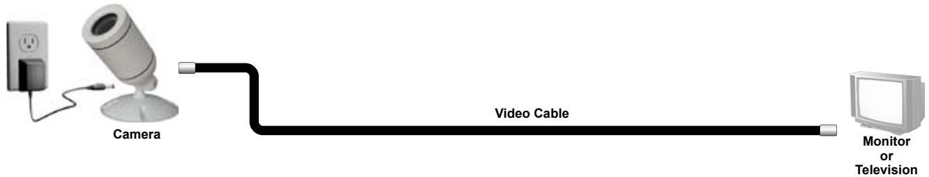
Figure 1 - Connecting the camera to a security monitor or standard television. Use the TV's composite RCA Video In jack and view through its video or line input. The picture will not be available on a channel.
